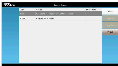
If need erase the fault codes, please exit the fault code interface to Function Selection Interface by click the button **[Back]**, Click **[Main page]** to exit to main interface
