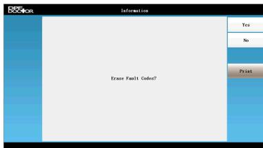
(2) Select **[ok]** to erase the fault code, select **[No]** to exit.
